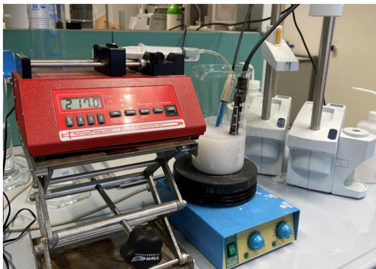
Figure 3. Lab-scale setup for reactive precipitation of \text{Mg}(\text{OH})_2 .
