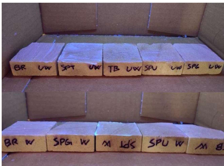
Fig. 3. Different application methods on limestones for C7 product. W=wet samples, on air application; UW=underwater application; BR=brush, SPT=spatula, TB=toothbrush, SPU=PVA sponge, SPG=sponge.
