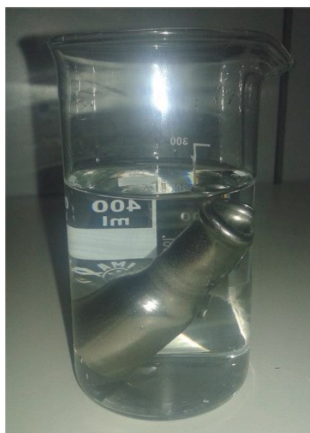
Figure 40: Experimental setup for the metal release test.
