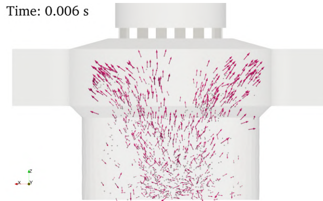
Figure 7.11: Direction of particle velocity at the beginning of the simulation (simulation T100).
