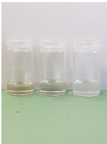
Figure 4.1.4. Electrolyte solutions 1:1 with PMMA's solutions: PMMA 996 on the left, PMMA 120 in the middle and PMMA 15 on the right.
