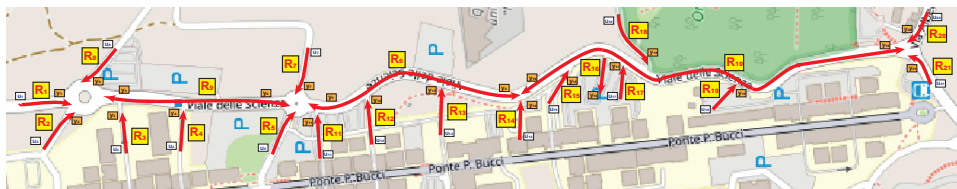
FIGURE 3.3: Example of a traffic compartmental system. Road schematic around the University of Calabria. R_i denote 21 potential sensor locations, u_i and y_i the vehicles entering and leaving the i -th link, respectively.
