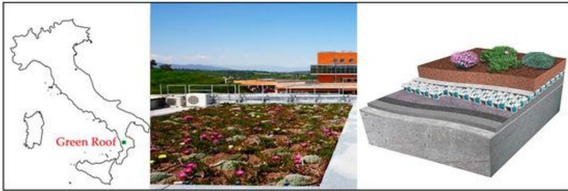
Figure 4.1: The experimental green roof (GR) located at the University of Calabria, Italy. A map of Italy, with the location of the green roof (left), the GR experimental site (middle), and an axonometric detail stratigraphy (right). All the figures were captured or created by the Urban Hydraulic and Hydrology Laboratory, University of Calabria, Italy (Palermo et al., 2019b).
