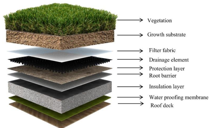
Figure 2.1: Green roof components (Vijayaraghavan, 2016).
