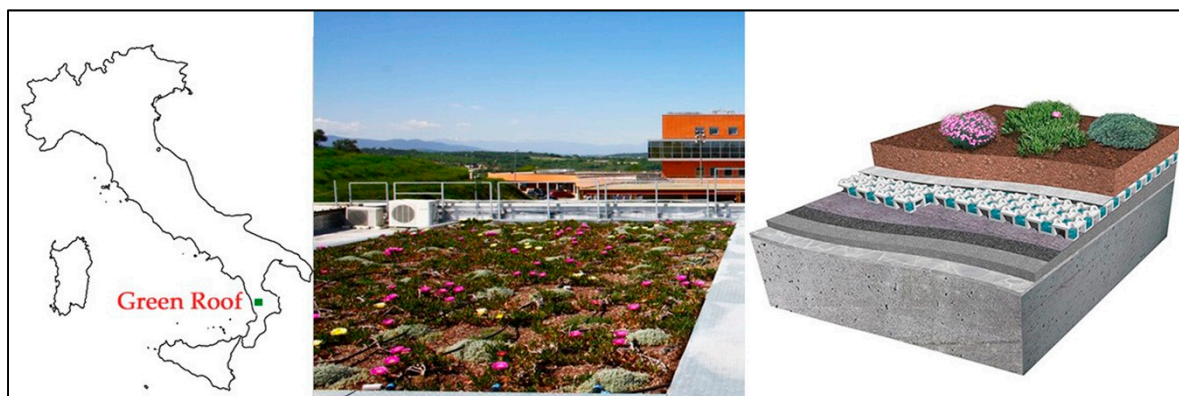
Figure 1. The experimental green roof (GR) located at the University of Calabria, Italy. A map of Italy, with the location of the green roof (left), the GR experimental site (middle), and an axonometric detail stratigraphy (right). All the figures were captured or created by the Urban Hydraulic and Hydrology Laboratory, University of Calabria, Italy.
