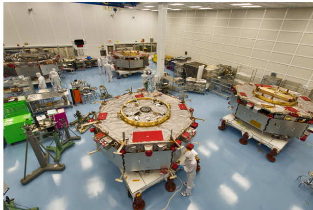
Figure 5.2: MMS four separate-view of all four spacecraft in the MMS Clean-room getting prepared for stacking operations. Photo credit: NASA/Chris Gunn
