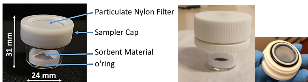
Fig. 3.12 PAS structure before (left) and after (right) improvements. The double cap system is also reported
