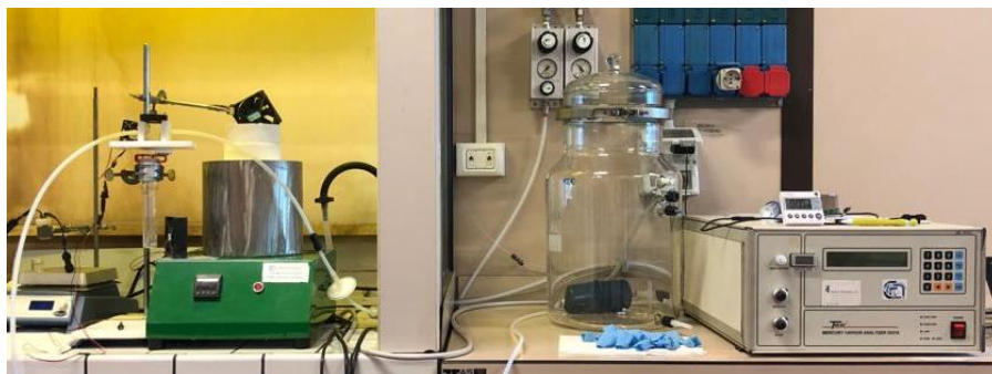
Fig. 2.3 Thermal desorption system for the analysis of passive samplers developed by CNR-IIA
