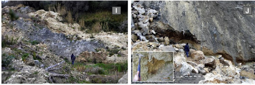
Figure 4.12 – Photos taken in the lower sector of the landslide: (I) chaotic mixture of yellowish-white limestone, ranging in size from sand to small blocks, and reworked blue marls of the flow tongue filling the valley bottom of the Scotrapiti Torrent; (J) particular of the flow tongue overlapping the in situ Tortonian sandstones. (From Borrelli et al. (2014))
