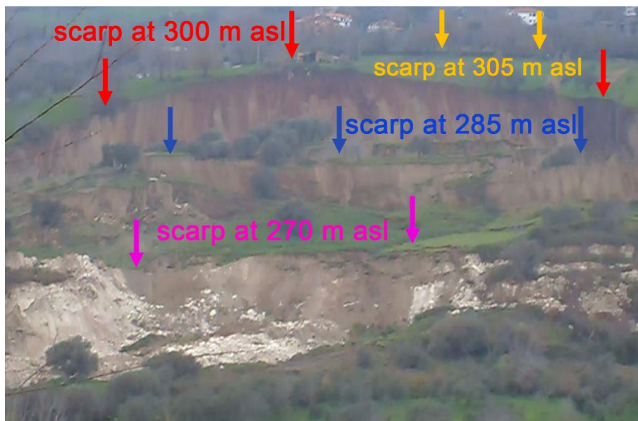
Figure 4.7 – Failure surfaces of the 15 February 2010 landslide. The pre-existing scarp at 305 m a.s.l. (indicated by the yellow arrows) was not involved in the failure process
