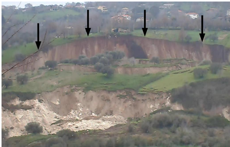
Figure 4.59 – Screenshot taken from a video filmed during the post-failure stage of the landslide, corresponding to the output plotted in Figure 4.57b (black arrows indicate the scarp at 300 m a.s.l.)
