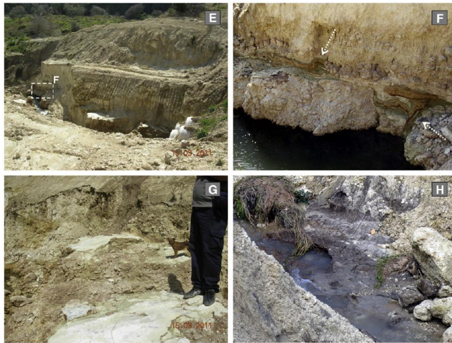
Figure 4.11 – Photos taken in the intermediate sector of the landslide: (E) large rock blocks of evaporitic limestone, little deformed, translated downstream; (F) laminated marl strata, interbedded inside the evaporitic limestone, stretched and deformed asymmetrically; (G) secondary sliding surfaces exposed on the remnant marl strata; (H) toe of the failure surface of the Maierato landslide daylighting (for about 20 m) in the terminal part of the intermediate sector. (From Borrelli et al. (2014))
