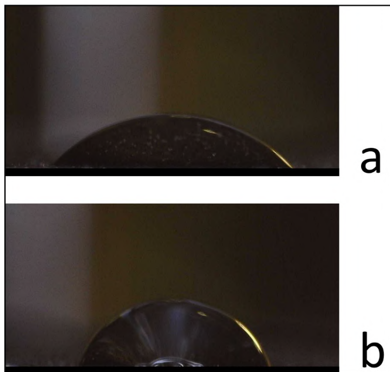
Figure S9. Average contact-angle value of: a) a SWCNT-BP ( \theta = 47.5^\circ \pm 0.5^\circ ) and b) a MTV-MOF/SWCNT-BP ( \theta = 78.5^\circ \pm 0.5^\circ ).
