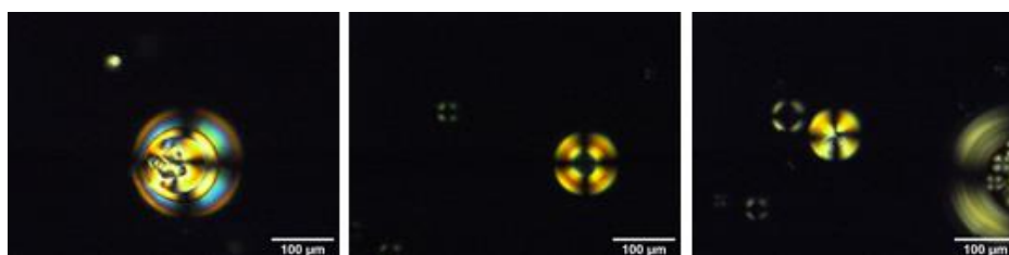
Figure 4.21: observation of the emulsion texture after 10 minutes (20x magnification)
