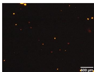
Figure 3.15: Homeotropic structure of the mixture in a cell with a 25µm thickness.
