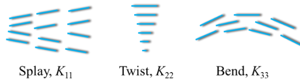
Figure 1.3 Schematic diagram of splay, twist and bend distortions in LCs, corresponding elastic constants are K_{11} , K_{22} and K_{33} .
