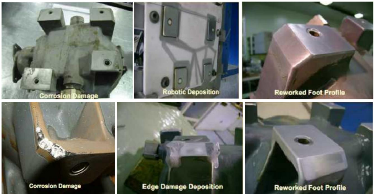
Fig. 1.24: Cold spraying restoration of corroded surfaces of an helicopter Seahawk gearbox unit [31]
