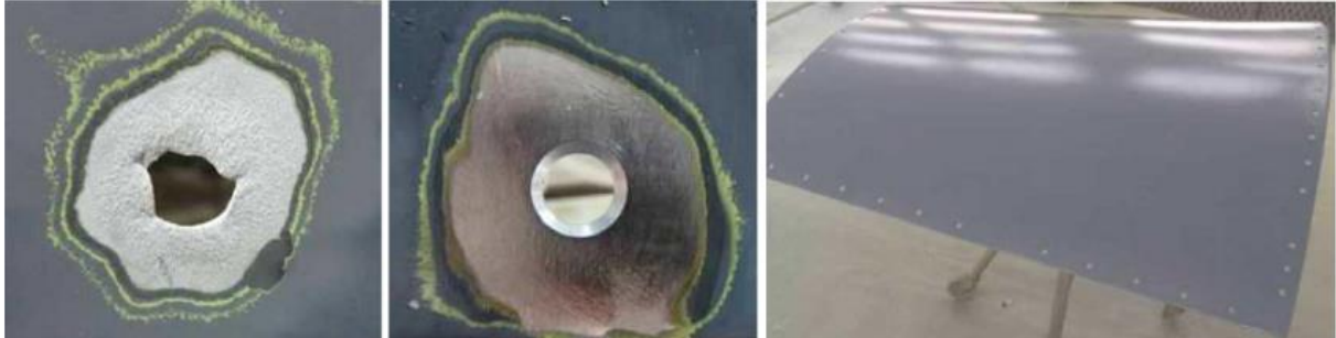
Fig. 1.25: Cold spray repair of fastener holes that enables a full restoration of a panel structure [32]
