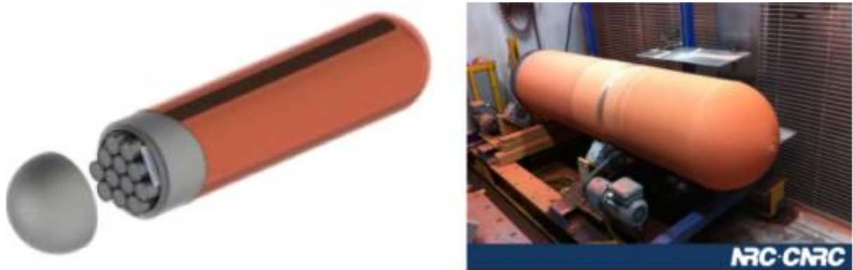
Fig. 1.21: Illustration of nuclear fuel container and copper cold sprayed prototype for a sustainable corrosion resistance [29]
