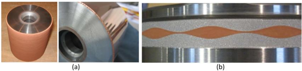
Fig. 1.22: Copper cold sprayed coating for automotive applications. Coating for printing rolls (a) and specifically shaped coating (b) [30]
