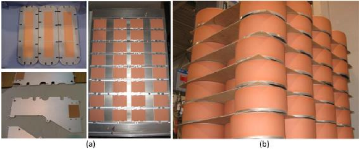
Fig. 1.23: Copper cold sprayed coating for power electronic heat sinks (a) and for refrigeration units (b) and mass production [30]
