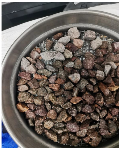
Fig. 1. Trentino porphyry used for the Boiling Test.
