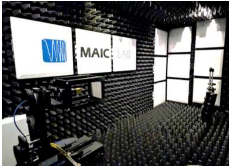
Figure 4-23 Dual-band dual-polarized M-FSS TA prototype mounted in the receiving mast of the anechoic chamber available at the MAIC-LAB, at the University of Calabria, Italy.
