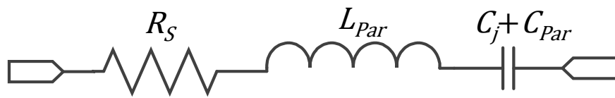
Figure 3-4 Equivalent circuit of the varactor diode including the parasitic effects of the package. ( L_{Par} = 0.4 nH, and C_{Par} = 0.06 pF)
