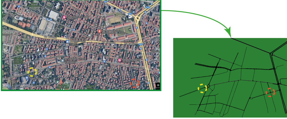
Figure 4.25: On the left, the URN from the A. Costa district in Bologna in Google Earth. On the right, the same URN in SUMO. The leader initial (yellow) and target (red) locations are highlighted.
