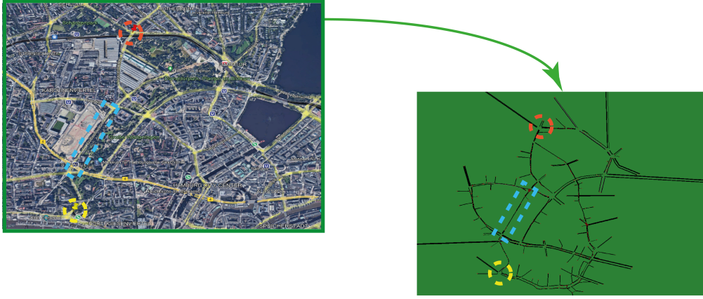
Figure 4.20: On the left, the URN from the city of Hamburg in Google Earth. On the right, the same URN in SUMO. The leader initial (yellow) and target (red) locations and the edge with traffic limitation (ciano) are highlighted.
