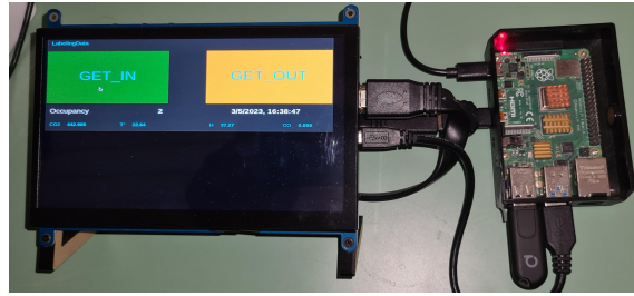
Figure 4.11: The touchscreen connected to the EDGE 1 Raspberry Pi.
