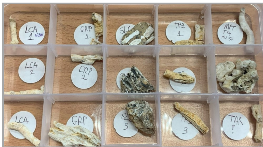
Figure 3. Some of the samples prepared for XRD screening.
