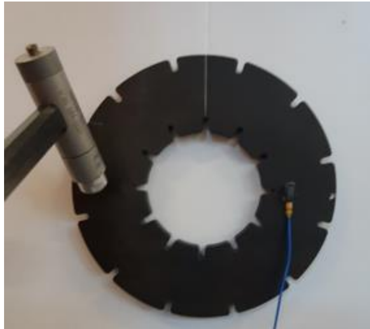
Figure 4. 10 Impact and acquisition points for the composite web.
