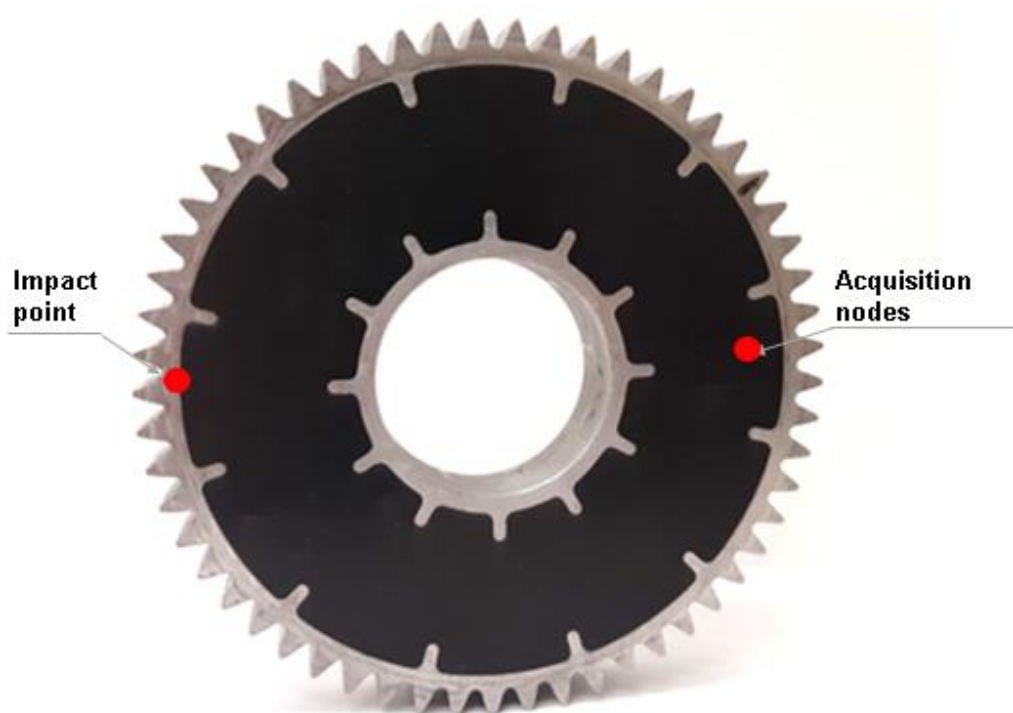
Figure 4. 18 Hybrid gear assembled by interference fitting.
