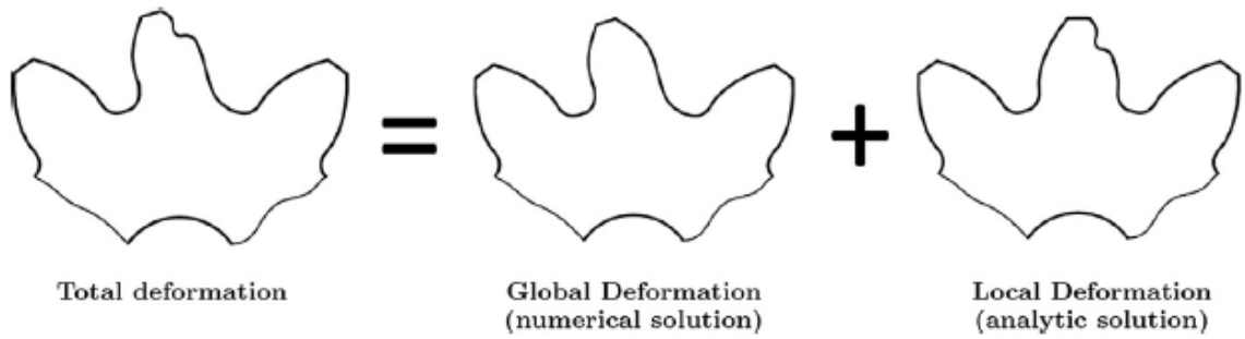
Figure 5. 9 Gear displacement field with hybrid FE analytical solution [83].
