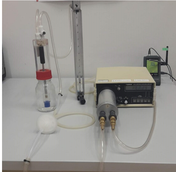
Figure 2.15: Water measurement with the emanometric technique at IRL. The blue porous stone in the bottle.
