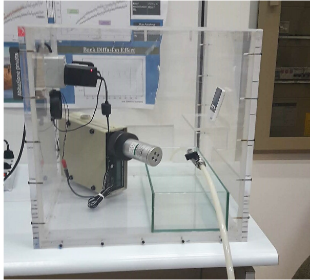
Figure 2.19: Experimental set-up for measuring radon concentration in water sample in a closed chamber.
