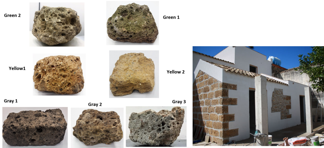
Figure 2.7: (Left) Samples of Lazio tuff with different colors, porosity, density, weight, volume and pumice stone inlays. (Right) Modern design of an Italian house, using volcanic tuff on the walls.
