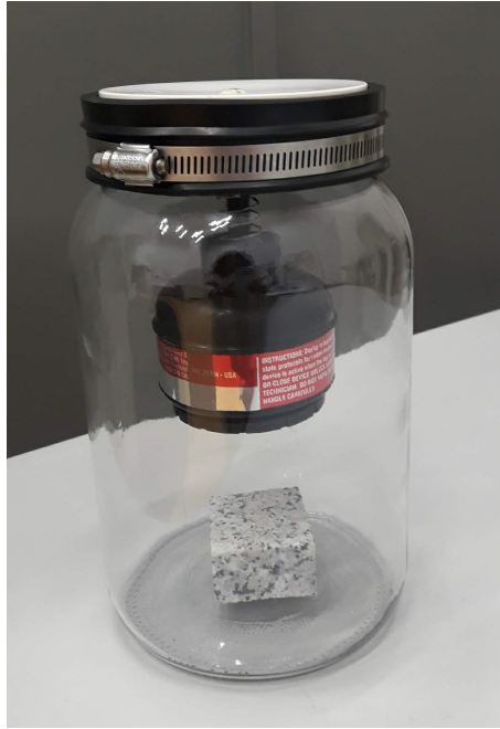
Figure 2.14: Radon exhalation measurement using the electret ion chambers technique.
