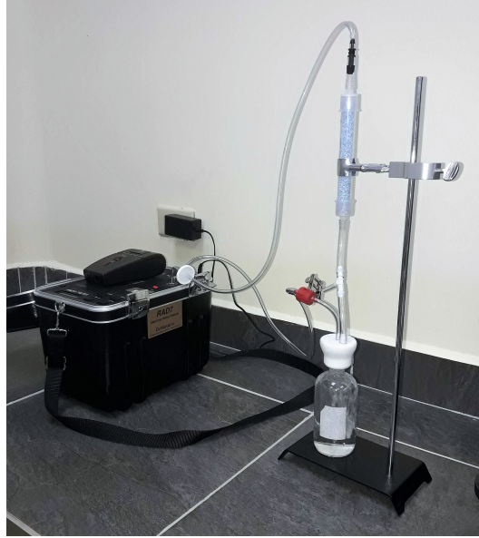
Figure 2.16: NTL emanometric apparatus: RAD7 monitor and DurrIDGE RAD H2O Rn kit.
