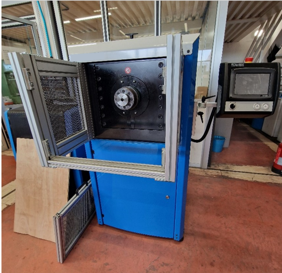
Figure 3.9: Photograph of the ad hoc designed and developed machine for SMA ring expansion.
