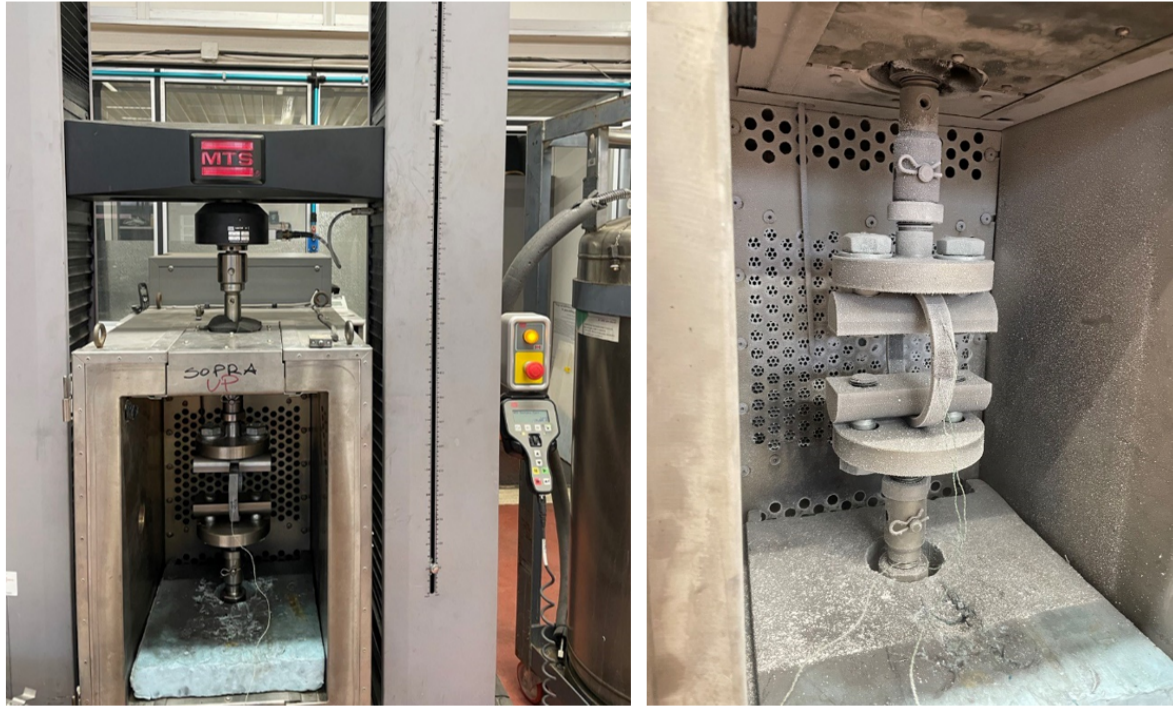
Figure 3.15: Machine and set up used for oval-shaped connectors tests.
