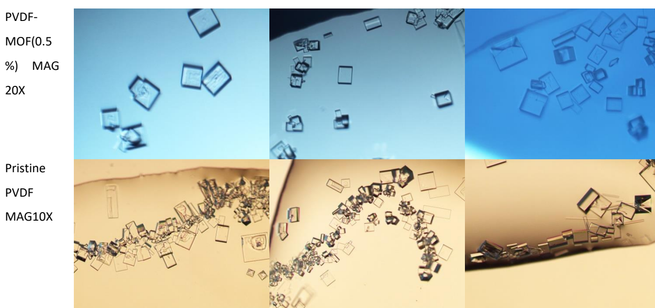
Figure 8.8 Pictures collected during the crystallization test with PVDF-MOF membrane at three different times.
