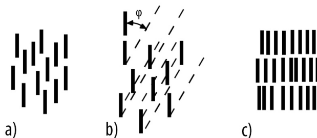
Figure 1: Structure of liquid crystals of the nematic a), cholesteric b), and smectic c) types.
