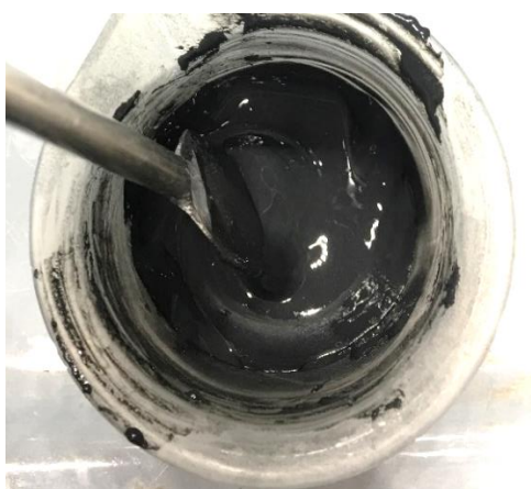
Figure 7.9 a). Slurry made from metakaolin, alkali activator and OAB
